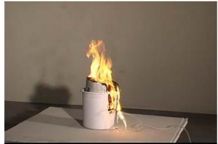
Figure 3.2-10. Trash container 2, 100 s after ignition
