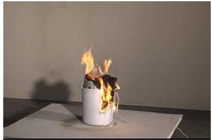
Figure 3.2-2. Trash container 1, 100 s after ignition
