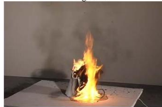
Figure 3.2-4. Trash container 1, 300 s after ignition
