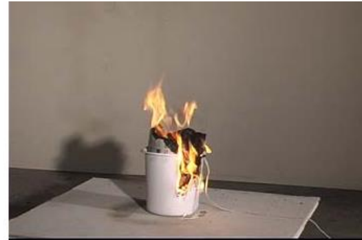
Figure 3.2-2. Trash container 1, 100 s after ignition
