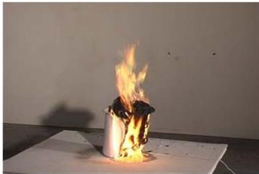
Figure 3.2-3. Trash container 1, 200 s after ignition
