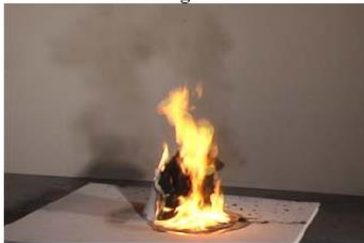
Figure 3.2-5. Trash container 1, 400 s after ignition
